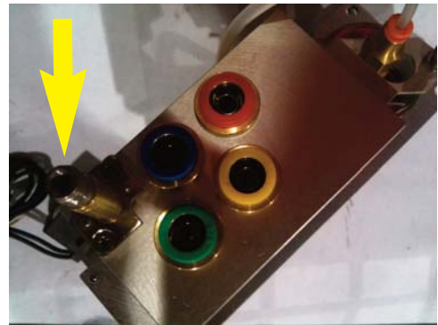
Solenoid Armature Replacement ( 2-screws )
