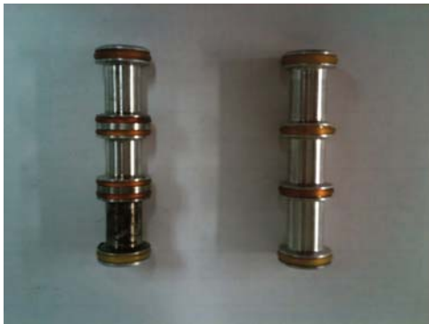
Spools ( Gen 2 on left and Gen 1 on right ) Gen 2 spools will work in Gen 1 kits, but Gen 1 spools will not work in Gen 2 kits.
