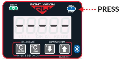
Press the MENU button and enter the new 5-digit PIN code using the 1, 2, 3, and 4 buttons. Press the MENU button again to save the code.
