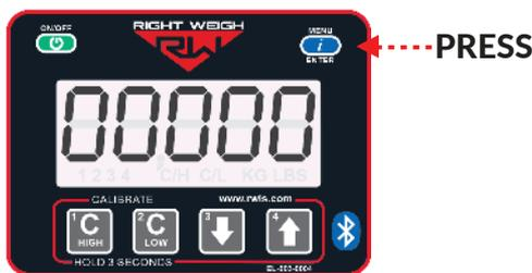
Press the MENU button and "00000" will display on the screen. Enter a 5 digit PIN code using the 1, 2, 3, and 4 buttons. Press the MENU button again to save the code.
