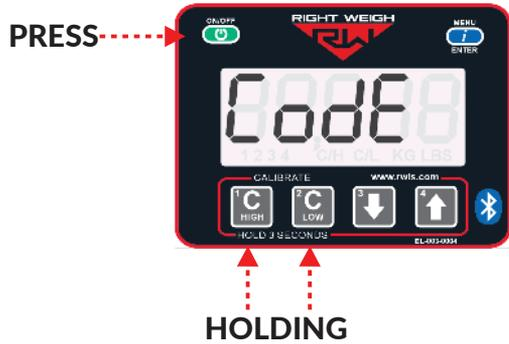
Press the MENU button and "-----" will display on the screen. Enter the previous PIN code. If the code entered is correct, the display will show "Good".
