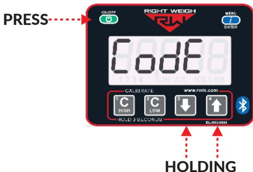
With the gauge off, hold both the C LOW and C HIGH buttons, then press the ON/OFF button and release all three.
